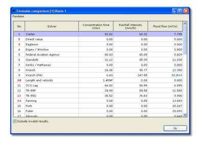
The methods that could not be solver due to insufficient data are marked with red. The highest value for the flood flow, regardless of the calculation method used, is marked with blue.
