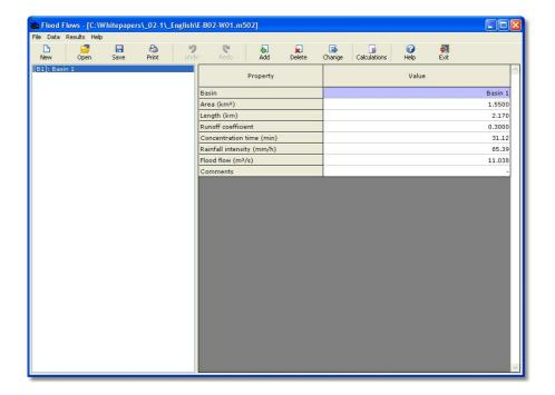
In order to compare the results of the selected calculation method with the results of all the other methods for calculating concentration times and flood flows, select **Results > Basins > Comparative Analysis** or hit **F3**:
