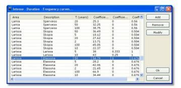
The basin is near Elassona so select the Elassona curve for a return period ( $\mathbf{T}$ ) of 50 years (which is an adequate period for a water drainage collector). Press  $\mathbf{Ok}$  twice to close the open forms.
