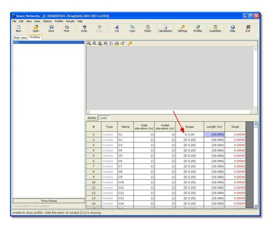
Based on auto-fill, the rest of the conduits are assigned the same shape. In their case, the name of the shape appears within curly braces.
