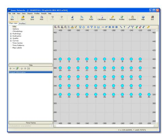
From the menu, select **Objects > Add > Conduit.** Holding down the **CTRL** key, click successively from junction to junction to create conduits according to the flow direction:
