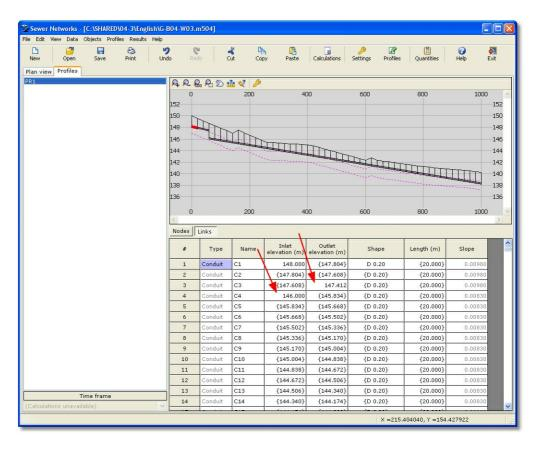
Alternatively, the program can put the conduit automatically to a specified depth. Select **Profiles > Automated branch design** from the main menu:
