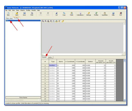
As displayed in the status bar, drawing the profile is impossible as critical information is missing. Click on the **Links** tab. To facilitate data input, from the menu select **Profiles > Stations:**
