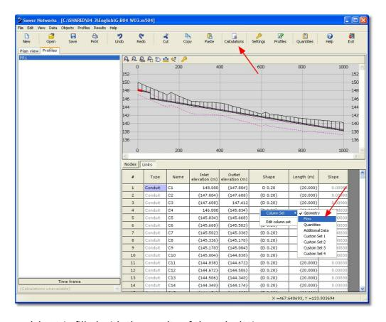
The spreadsheet is filled with the results of the calculations:
