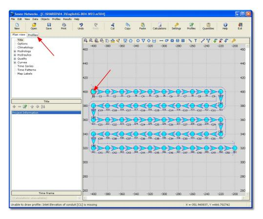
We will make the safest assumption that all the runoff area ends up in the first junction. Double-click on junction **J1** in the plan view to display its properties:
