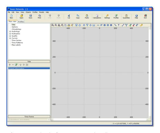
In case of sewer networks, the flows are in general small. It is convenient to use L/s instead of  $m^3/s$ . From the menu, select **Data > General Data > General** and select **L/s** as flow units:
