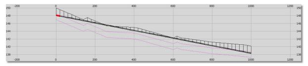
It is evident that we need to lower the conduit. We will use a drop inlet between the third and fourth conduit. Double-click on the third conduit **in the profile sketch.** The corresponding line will be highlighted in the spreadsheet.
