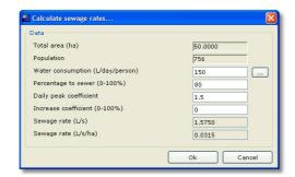
Typical values include **water consumption** equal to 150 L /day /person, **80%** of the water consumption ends up in the sewer and the **daily peak coefficient** is set equal to **1.5.** Press **Ok** to accept the calculated values of **sewage rate** and return to the previous form:
