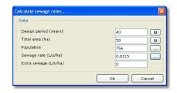
Assuming that the **extra sewage** is equal to 10% of the sewage rate, enter **0.0031** L /s /ha in the corresponding field. Press **Ok.**
