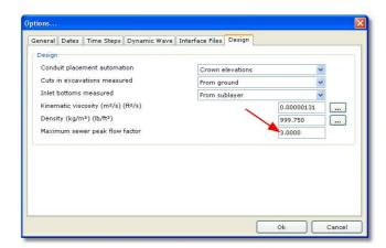
According to Greek Regulations, the maximum sewer peak flow factor cannot exceed 3.0.
