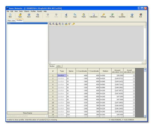
Note that the cells in which you typed a known ground elevation do not have curly braces. On the other hand, the unknown ground elevations are auto-filled based on upstream and downstream known values and, thus, they are displayed within curly braces.
