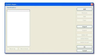
Press **Add**. In the **Shape data** tab, input the data of a circular shape made of PVC with internal diameter of 0.2m:
