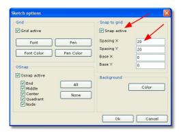
Check **Snap active** and set the **spacing X** and **spacing Y** equal to 20. Press **Ok.**
