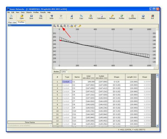
The profile sketch is a very useful design tool. Assuming that the minimum acceptable backfill depth is 1.5m and the maximum acceptable excavation depth is 3m. Right-click on the profile sketch. From the menu, select **options**. The following form appears:
