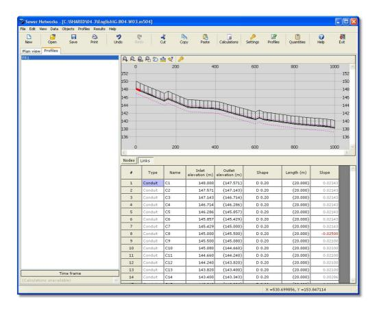
Note that the program performs a host of checks regarding the slopes, maximum/ minimum velocities, capacities etc. All fields that fail to pass a check are displayed in a different (but customizable) color. The default color that is used in these cases is red. Thus, it is obvious that the slope of the conduit C8 is negative.
