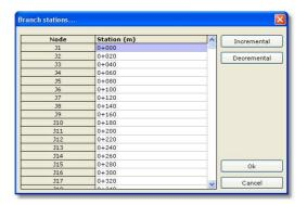
Press **Incremental.** The program assign the correct stations to junctions according to the distances in plan view. Press **Ok.**
